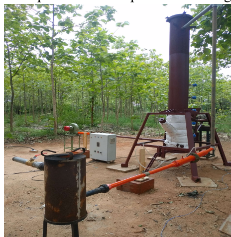
Figure 1: Fluidized bed gasifier for leafy biomass
