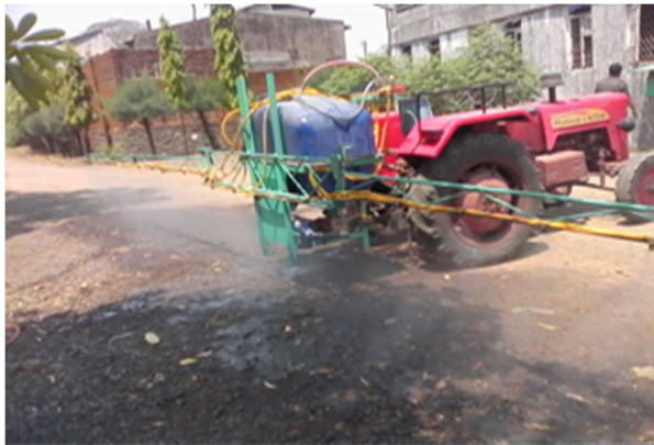
Figure 4: Modified hydraulic boom sprayer
