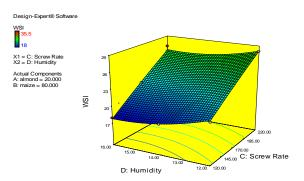
Figure 2: Effect of humidity and the rotation screw rate of the helix on the properties of water solubility
