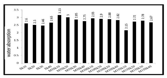
Figure 8 - water absorption of samples in the first and second phases
