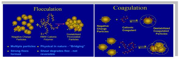
Figure 1: The chemical process of separation of particles from liquid (4)
