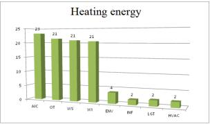
Figure 4- the diagram of heating energy consumption in improving different modes (KWh/m<sup>2</sup>/yr)
