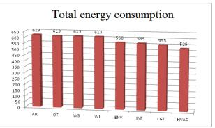
Figure 3- the diagram of comparing total fuel consumption (gas and electricity) inimproving different modes (KWh/m<sup>2</sup>/yr)
