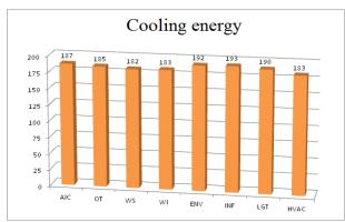
Figure 5- the diagram of cooling energy consumption in improving different modes  $(KWh/m^2/yr)$
