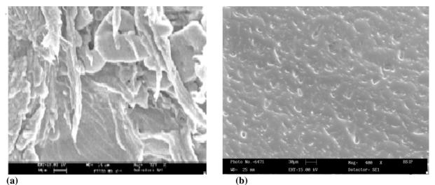
Fig.1.Scanning electron micrograph of (a) polymeric film of batch F6S0; (b) polymeric film of batch F6S25
