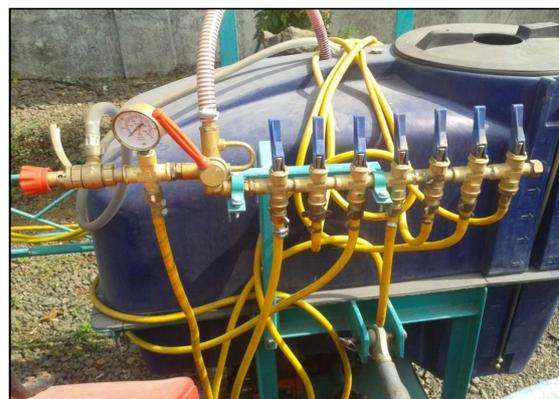
Figure 2(b): Set-up 2 Six control valve assembly
