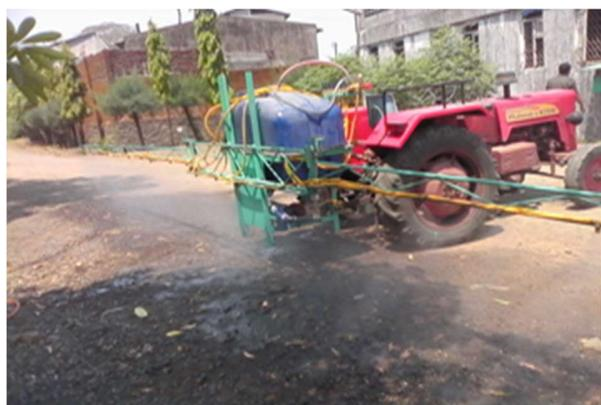
Figure 4: Modified hydraulic boom sprayer
