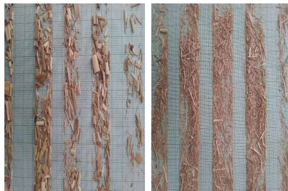
Figure 1a: Raw Material for Briquettes- Chopped Straw Figure 1b: Raw Material for Briquettes- Shredded Straw). Note: The smallest graph paper square size- 1mm x 1mm.
